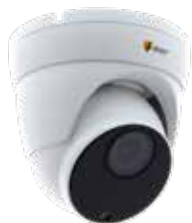
IED-64M2812MBA | Art.-Nr. 218033 1/3" Network Dome, Day&Night, 2592x1520, H.265, Infrared, 2.8-12mm, PoE, IP66
