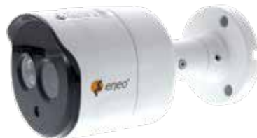
IEB-54F0028M0A | Art.-Nr. 225714 1/3" Network Camera, Day&Night, 2592x1520, H.265, Infrared, 2.8mm, PoE, IP66
