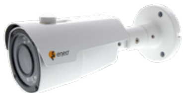
IEB-64M2812M0A | Art.-Nr. 218032 1/3" Network Camera, Day&Night, 2592x1520, H.265, Infrared, 2.8-12mm, PoE, IP66
