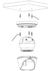
**Step 5:** To position the camera, align it with the triangle symbol and turn it in the direction shown in the illustration.
