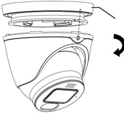
**Step 4:** Drill the holes marked on the mounting template and use plugs and screws to secure the base.
