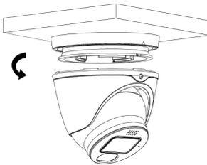
**Step 6:** Align the camera at the desired angle and tighten the screw again to secure the camera.
