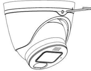
**Step 3:** Turn the base and align the screw with the triangle symbol, then remove the camera as shown in the illustration below.
