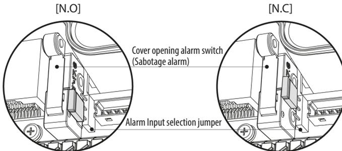
For Cover Opening Alarm, please go to SETUP> Event Rules> Event Processing> Add Event Trigger should be set to "Alarm In" and then Event Action should be set as available options
