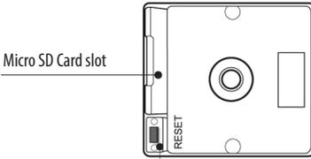
IP Reset (Default) : pressing for 5~8 seconds resets all parameters to original factory settings.
