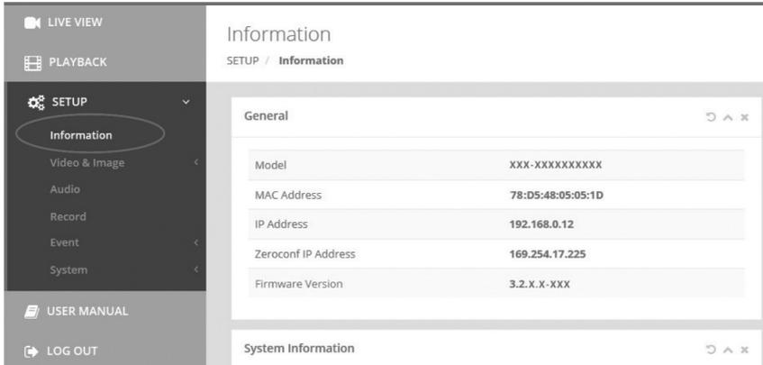
The screenshot shows the 'Information' page in the camera's web interface. The left sidebar contains navigation options: LIVE VIEW, PLAYBACK, SETUP (with a gear icon), USER MANUAL, and LOG OUT. The 'SETUP' menu is expanded, and 'Information' is selected and circled. The main content area is titled 'Information' and shows 'SETUP / Information'. Below this, there are two sections: 'General' and 'System Information'. The 'General' section contains a table with the following data:
