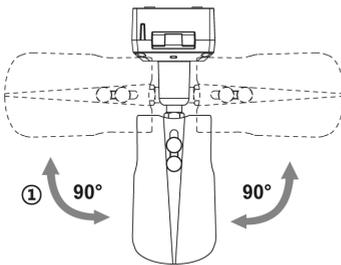
2. Tilt limit: Tilt is limited to 0°(2°) min ~ 90° max. for wall(ceiling) installation respectively with reference to the wall(ceiling) when the inclination of camera module is 0°, that is, the image is aligned horizontally.
