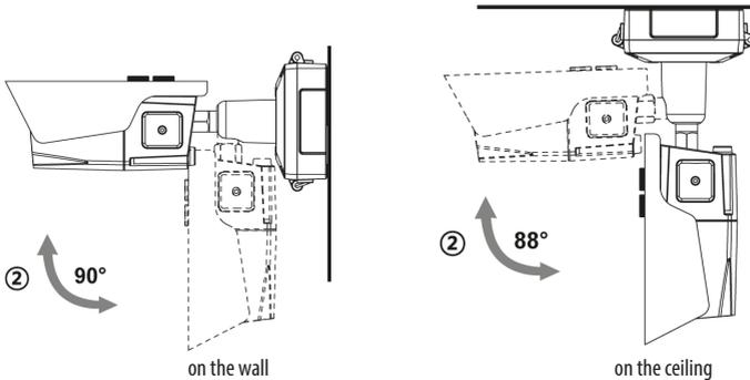
3. Inclination limit (Horizontal image alignment): Inclination limited to +/-90° max.
