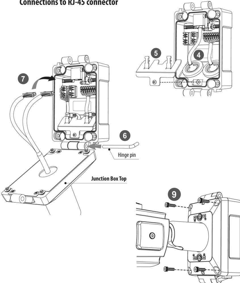
10. Set the camera's orientation and tighten the Lock/Unlock screws using hex wrench.
