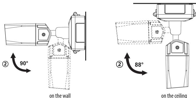
3. Inclination limit (Horizontal image alignment): Inclination limited to  $+-90^\circ$  max.
