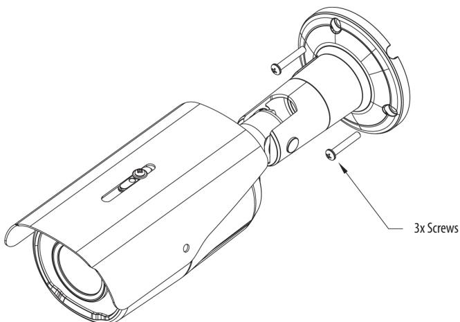
**CAUTION:** Adjusting the position of the camera after installation could potentially damage the cable.
