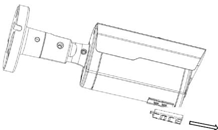
4. Adjust zoom and focus using flathead screw driver.
