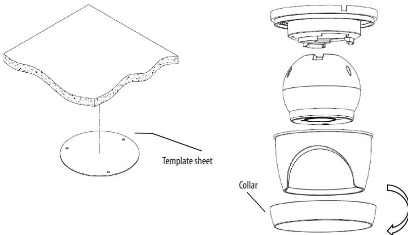
3. Fix the base of the camera with the three screws provided in the accessory kit.
