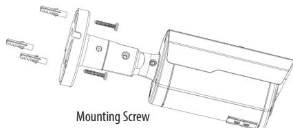
2. Adjust the camera angle and tighten the mount using the L-wrench.
