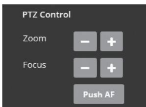
Used to adjust zoom/focus manually or one-push focus automatically.
