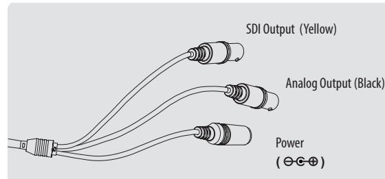
**i** Please use the cable as provided with camera. If camera cable is cut and re-wired, the transmission distance of video can be reduced. Especially SDI cable should not be cut because it requires detailed wiring job and affects the transmission distance.
