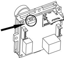
Follow the instructions below to reset the network camera to the factory default settings using the Reset button.
