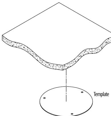
1. Paste the template sheet in place at the proper position.
