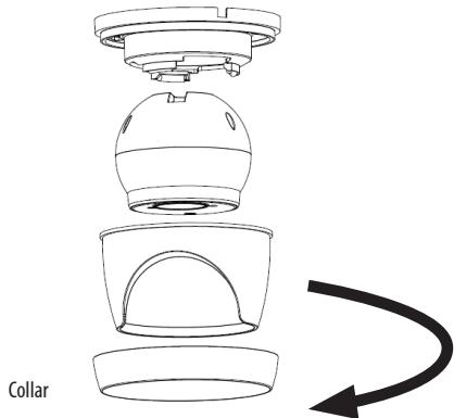
2. Remove the collar off the camera by rotating it down.
