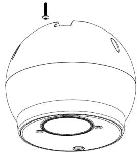
3. Fix the base of the camera with the three screws provided in the accessory kit.
