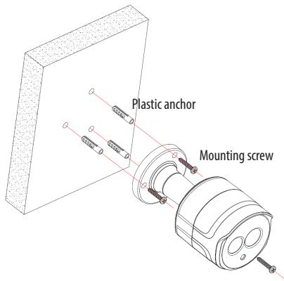
To mount the bullet camera, fix the base of the camera with the three screws provided in the accessory kit.
