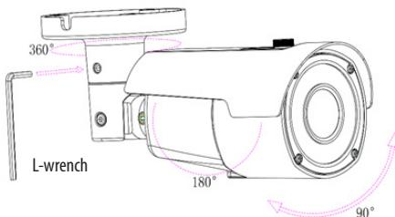
2. Adjust the camera angle and tighten the mount using the L-wrench.
