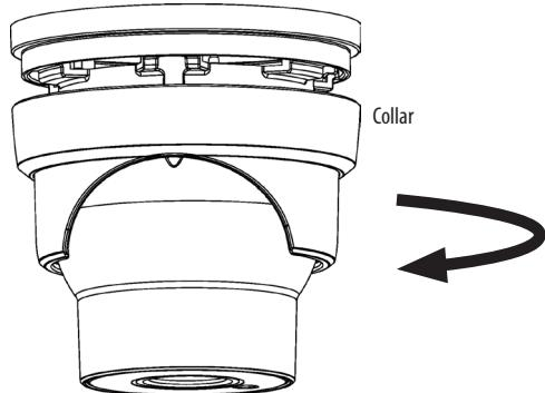
2. Remove the collar off the camera by rotating it down.
