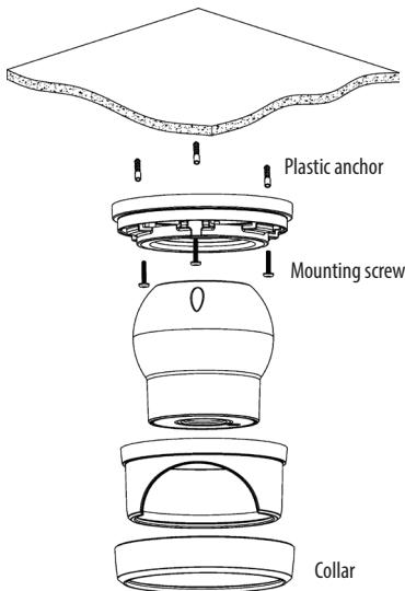
3. Fix the base of the camera with the three screws provided in the accessory kit.
