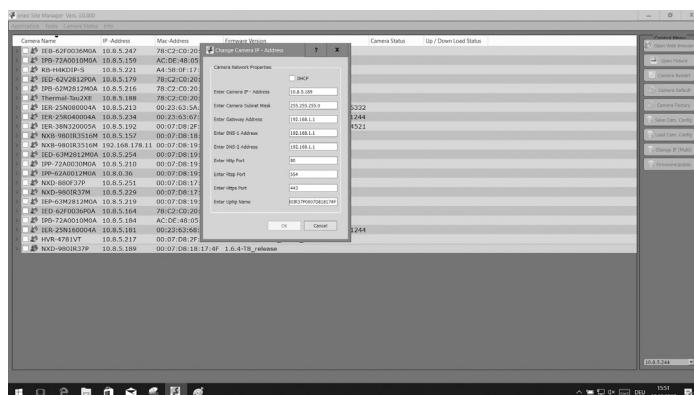
Select the „Set IP Address [dhcp / static]“ option to open a window for setting the camera as IP properties. When you are done click the „OK“ button to update the camera settings.
