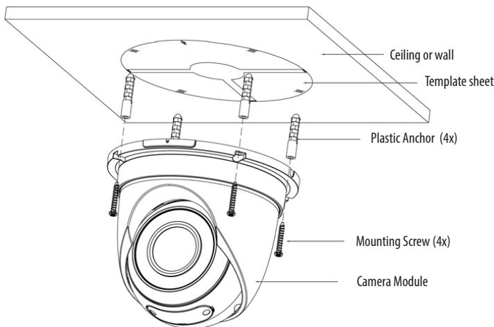
1. Make screw holes on the ceiling using the supplied mounting Template Sheet.
