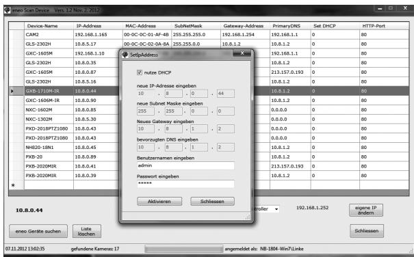
Select the „Editing the camera IP address“ option to open a window for setting the cameras IP properties. When you are done click the „Activate“ button to update the camera settings.
