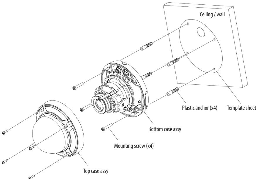
4. Put the front of the housing on the bottom case and thighten the 4 torx screws.
