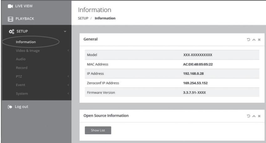
The screenshot shows the camera's web interface. On the left, a sidebar menu is visible with options: LIVE VIEW, PLAYBACK, SETUP (selected), and Log out. Under the SETUP menu, 'Information' is highlighted. The main content area is titled 'Information' and shows the following details:
