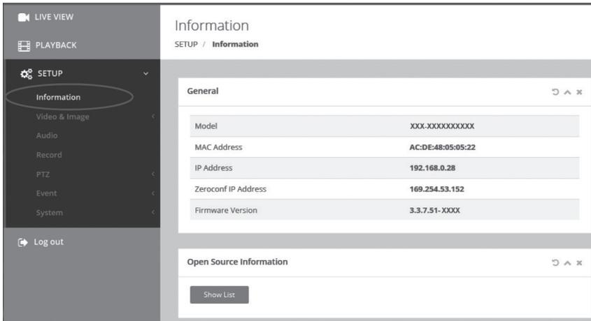
The screenshot shows the 'Information' page in the camera's setup menu. The left sidebar has 'SETUP' expanded, with 'Information' highlighted. The main content area is titled 'Information' and includes a breadcrumb 'SETUP / Information'. There are two expandable sections: 'General' and 'Open Source Information'. The 'General' section contains the following data:
