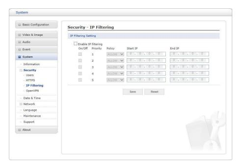
Checking the **Enable IP address filtering** box enables the IP address filtering function. Up to 256 IP address entries may be specified (a single entry can contain multiple IP ad- dresses). Click the **Add** button to add new filtered addresses.
