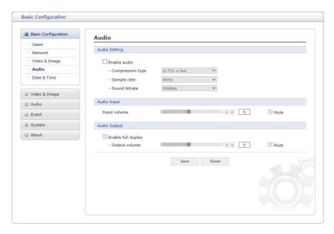
The network camera can transmit audio to other clients using an external microphone and can play audio received from other clients by attaching a speaker. User can setup and change setting of Audio in this page.
