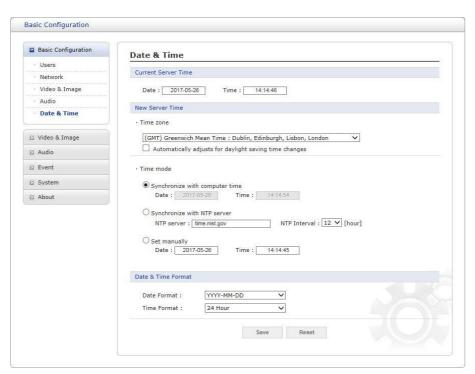
User can set time directly or assign time server to get the current time, as well as determine Date & Time format in this page.
