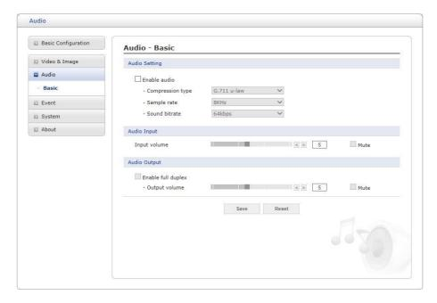
The network camera can transmit audio to other clients using an external microphone and can play audio received from other clients by attaching a speaker. The Setup page has an additional menu item called Audio, which allows different audio configurations, such as full duplex and simplex.
