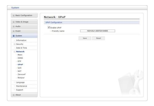
The network camera includes support for UPnP. UPnP is enabled by default, so the network camera is automatically detected by operating systems and clients that support this protocol. Enter a name in the Friendly name field.
