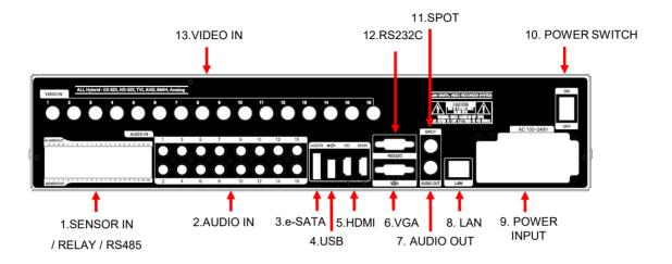
1. **SENSOR IN**: This terminals can be connected to external sensors.
