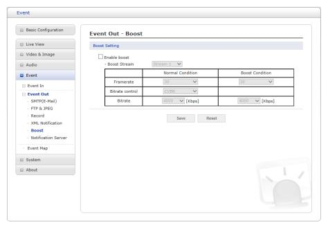
The Boost feature is used in conjunction with event detection. When this feature is turned ON, the Frame rate and Bit rate in the boost condition can be set to a different value than the ones in the normal condition field. When an event is detected, the camera will boost the Frame rate and Bit rate from the normal condition to this boosted level for the duration of the event.
