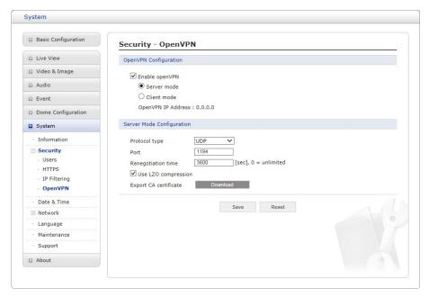
OpenVPN is a Virtual Private Network using OpenSSL authentication. User can set the camera in either Server mode or Client mode.
