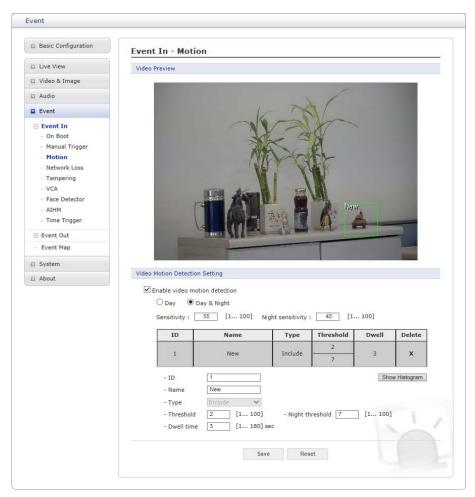
This option makes use of the motion detection function with 16 programmable areas, 8 **Include** and **Exclude** zones each.
