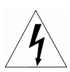
The lightning flash with arrowhead symbol, within an equilateral triangle, is intended to alert the user to the presence of uninsulated "dangerous voltage" within the product's enclosure that may be of sufficient magnitude to constitute a risk of electric shock to persons.
