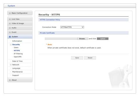
For greater security, the network camera can be configured to use HTTPS (Hypertext Transfer Protocol over SSL (Secure Socket Layer)). Then all communication that would otherwise go via HTTP will instead go via an encrypted HTTPS connection.
