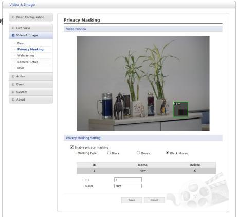
The privacy masking function allows you to mask parts of the video image to be transmitted. You can set up to eight privacy masks and the color of privacy masks is black.
