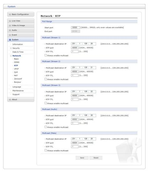
Create a setting for sending and receiving an audio or video on a real-time basis. These settings are the IP address, port number, and Time-To-Live value (TTL) to use for the media stream(s) in multicast H.264 format. Only certain IP addresses and port numbers should be used for multicast streams.
