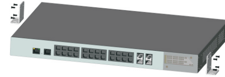
Figure 2-3 Hangers installation diagram
