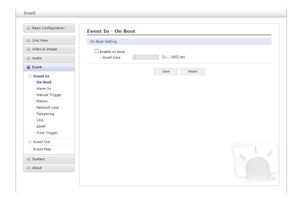
This is used to trigger an event every time the network camera is started. Se-
