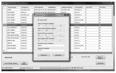
Select the "Editing the camera IP address" option to open a window for setting the cameras IP properties. When you are done click the "Activate" button to update the camera settings. For further information, please refer to the eneo Scan Device Tool Quick Start Guide.
