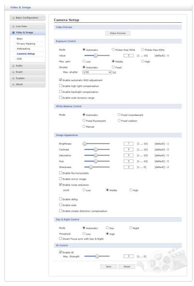
In this page, user can setup Exposure Control, White Balance Control, Image Appearance, and Day & Night control.
