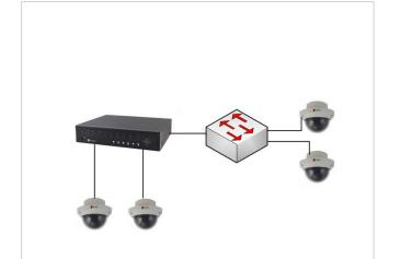
Preconfiguration 1x Network Video Recorder with more than 16 IP cameras
