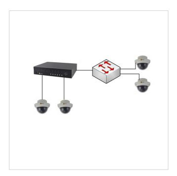
Preconfiguration 1x Network Video Recorder with up to 16 IP cameras
