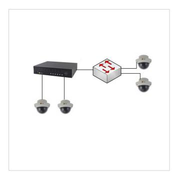
Preconfiguration 1x Network Video Recorder with up to 8 IP cameras
