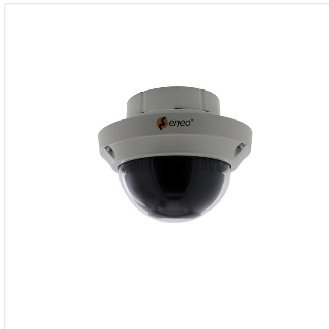
1/2,8" HD Dome Fix, Day&Night 3840x2160, Infrared, WDR, 2,7-13,5mm, 12/24V, IP67
